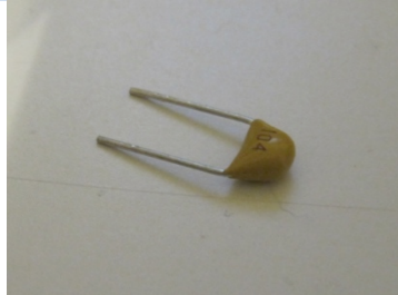
100nF capacitor (marked 104)
